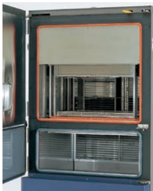
TSD Test areas (top: high temperature chamber bottom: low temperature chamber)
