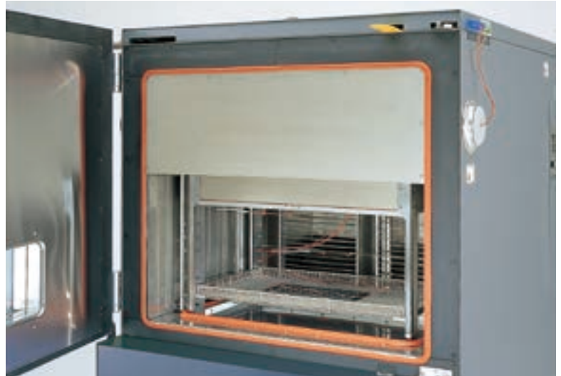
TSD Specimen temperature measurement (specimen temperature input standard equipment: 2 locations) (optional: 3 locations)
